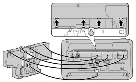
2. Fasten the wall mounting adaptor to the base with 1 screw. (Recommended torque: 0.4 N⋅m [4.08 kgf⋅cm] to 0.6 N⋅m [6.12 kgf⋅cm])
