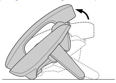
1. Tilt the stand in the direction indicated while pushing the PUSH mark with both hands as shown until it locks into the high position (A).
